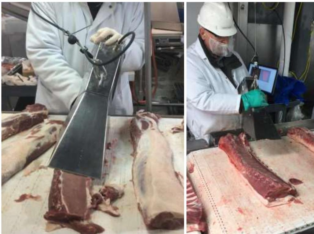
Figure 2. VQG operation on two different loin boning lines. In both cases, the operator is on the same side of the conveyor as the posterior end of the loins are oriented toward. Movies are available at: [http://www.eplusv.de/files/USMARC/VQG Movie Trimmed strap-off loins.mp4](http://www.eplusv.de/files/USMARC/VQG%20Movie%20Trimmed%20strap-off%20loins.mp4) and [http://www.eplusv.de/files/USMARC/On-line Pre-Trim VQG.MOV](http://www.eplusv.de/files/USMARC/On-line%20Pre-Trim%20VQG.MOV)
