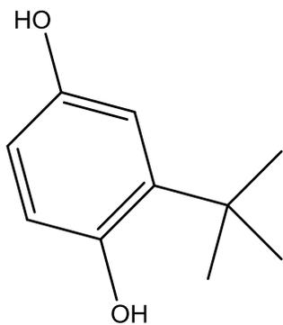
Figure 1. Structure of tertiary butylhydroquinone (TBHQ).
