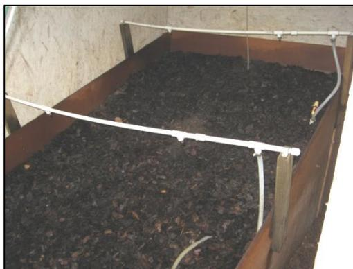
Figure 3. Biofilter inside of an enclosure, with a new four-nozzle hydration system.
