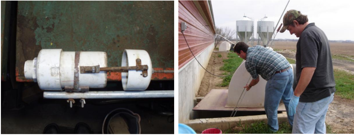
Figure 1. Pit slurry sampler used to collect slurry from deep pit swine operations. The sampler is lowered to depth and a rod is pulled that opens the sampler. The rod is connected to the cap and goes through the PVC capsule to a rubber stopper in the bottom of the PVC capsule. Manure enters through the bottom and top. Once full the sampler is closed by pushing the rod.
