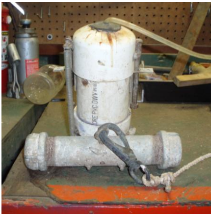
Figure 2. Pneumatic sampler for sampling above ground slurry tanks and the bottom of lagoons. The unit is lowered into the tank from the top/surface by rope (clipped to the weight). The weight allows the sampler to settle through the solids to the bottom. Once at the desired depth, water is forced down the hose and into a syringe inside the PVC sample container. As the syringe fills with water, the end cap is forced open and manure slurry enters the PVC capsule. The water is withdrawn (closing the end cap) and the unit is pulled back up to the top of the tank. Springs attached to the cap and side help to close the container.
