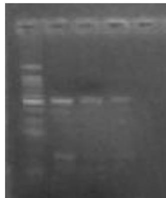
Figure 3: Slab gel image of a 100000:1 dilution of initial template by amplifying on the on-chip device.
