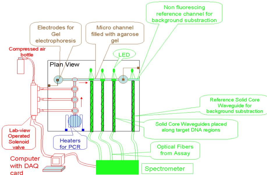
Figure 1. Schematic of the overall DNA assay units
