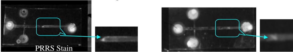
Fig. 6(a) Trial 1: Capillary electrophoresis on a chip (b) Trial 2: Capillary electrophoresis on a chip.
