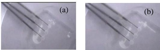
Figure 4: (a) and (b) Spanshots of the fluorescence dye flowing through the micro-channel taken at 4 secs. interval.
