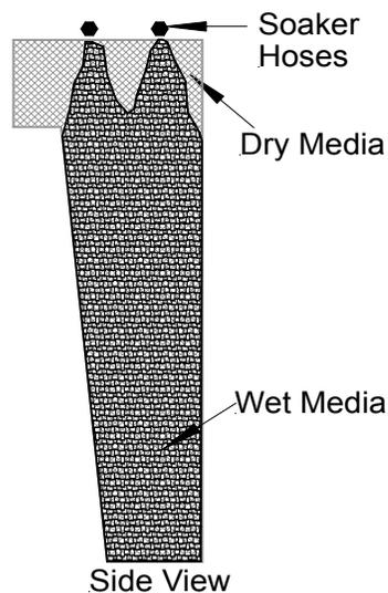
**Figure 4. Moisture profile with soaker hose on biofilter top.**
