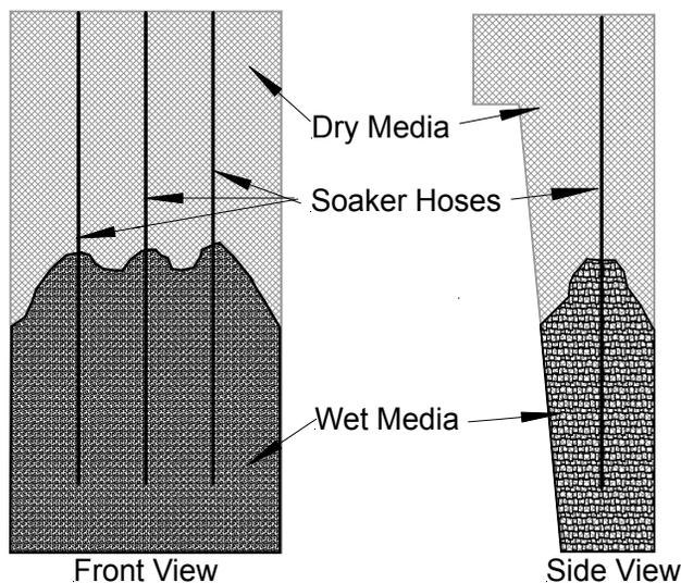
**Figure 3. Moisture profile with vertical soaker hoses.**
