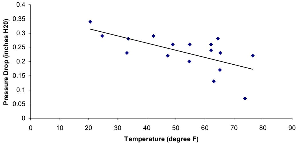
**Figure 5: Pressure Drop Measured vs. Average Daily Temperature for the day it was measured.**
