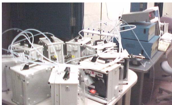
Figure 2- Lab setups for evaluation of SPM performance in measurement of H 2 S and NH 3 .
