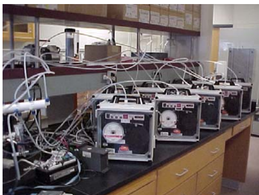
Figure 2- Lab setups for evaluation of SPM performance in measurement of H 2 S and NH 3 .
