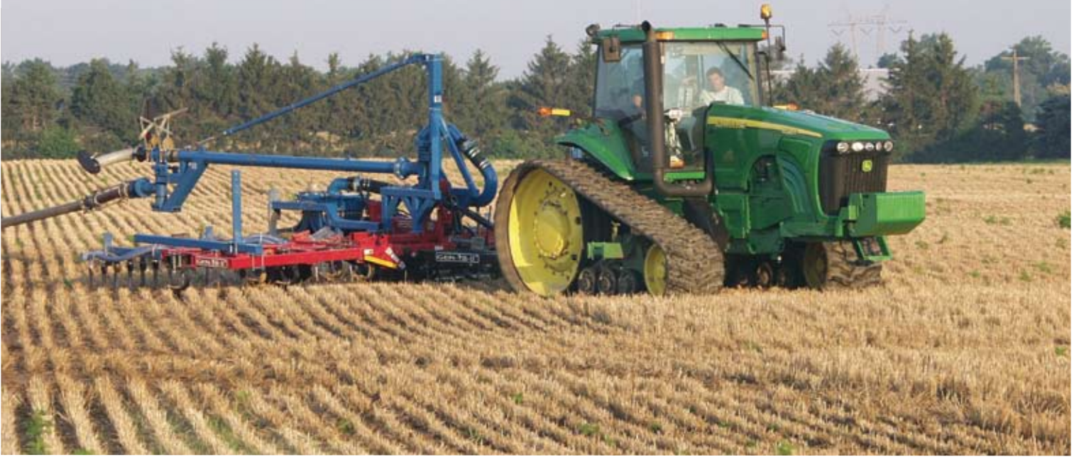
Drag line transports effluent to applicator
